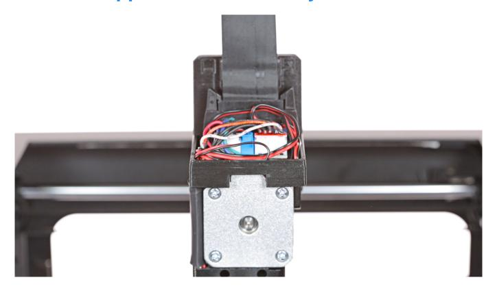
Attach the extruder upper cover to the extruder.
