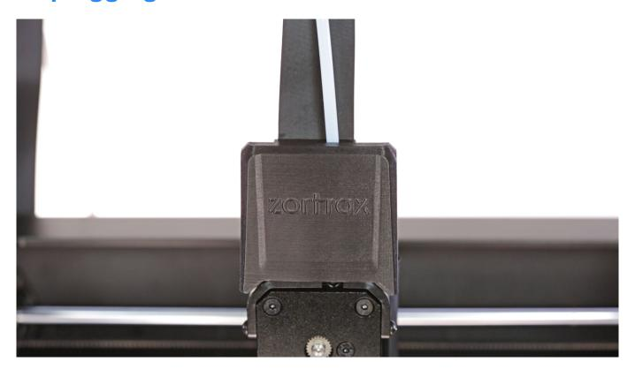
Detach the material guide and unplug the extruder cable.
