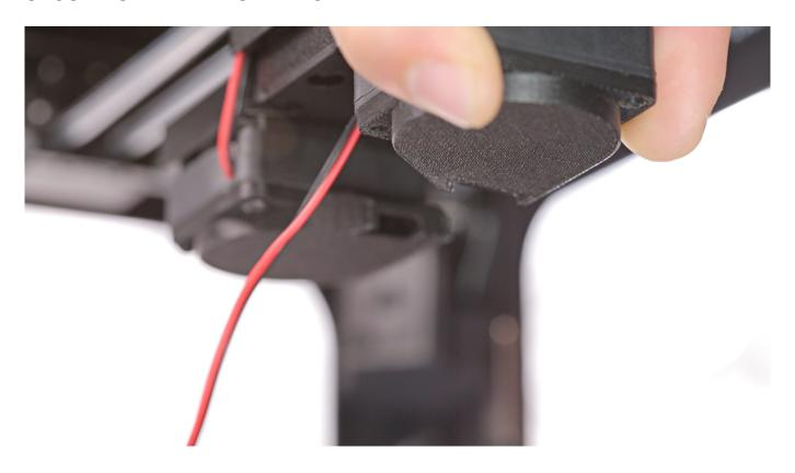
Secure the extruder lower fan with the two screws.
