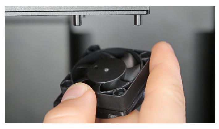
Place the distance piece on the extruder lower fan. Install the fan under the heat sink.
