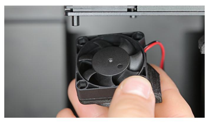
Place the distance piece on the extruder lower fan. Install the fan under the heat sink.
