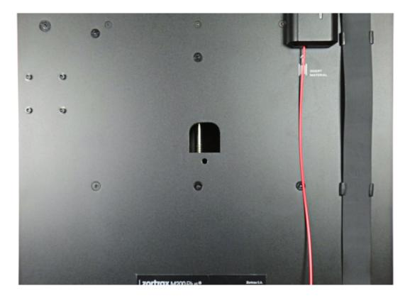
Attach the spool holder together with the spool to the back of the printer.
