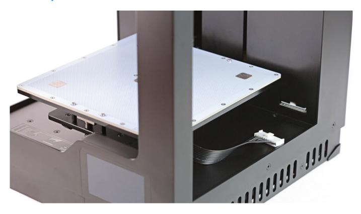
Plug the heatbed cable into the Z-axis cover.
