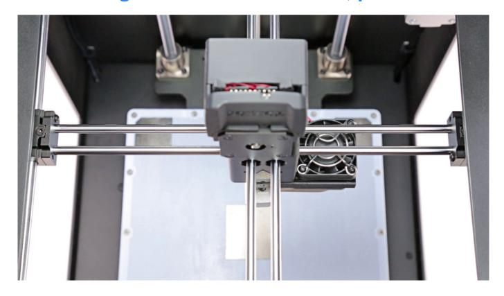
Unscrew the other screw that secures the axis block cover on each block.
