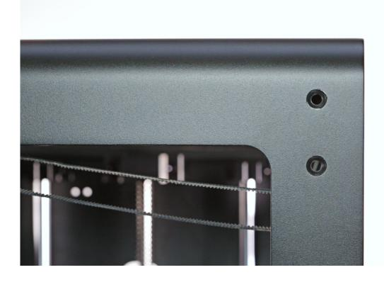
Secure the other self-aligning bearing of the axis that holds the lower long belt.
