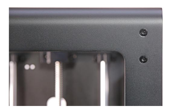
Unscrew the self-aligning bearing of the axis that holds the lower long belt to be replaced. Use a wrench or pliers to hold the nuts of the screws.
