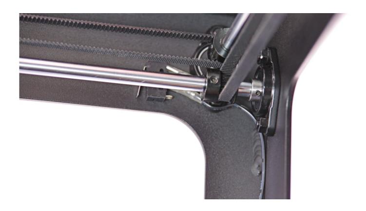
Loosen the screws on the self-aligning bearings on the axes that hold the lower long belt.
