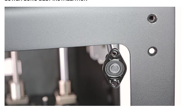
Put the new lower long belt on the axes that hold it.
