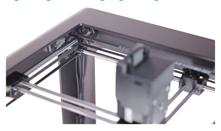
Tighten the screws that secure the self-aligning bearings on both sides of the housing.
