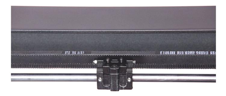
Unscrew the screw that secures the belt tensioner on the belt to be replaced and remove the belt from the block.
