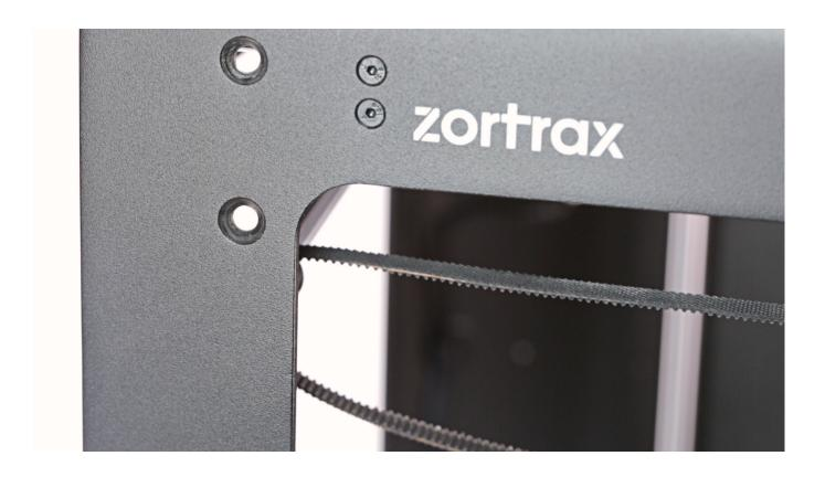
Remove the lower long belt from the axes that hold it.
