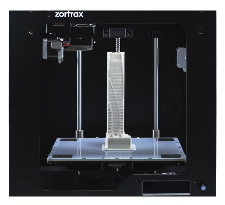
Once the printing process has been finished, leave the model on the platform for about 30 minutes to let it cool off. This will make it easier for you to remove your print from the platform. Also, you will be able to remove the raft and support structures from the model more easily.
