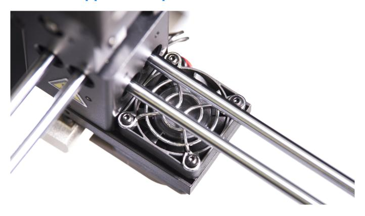
Check if the extruder upper fan is operating properly. A faulty fan can cause Z-PLA Pro to overheat which can have a negative influence on the printing process.
