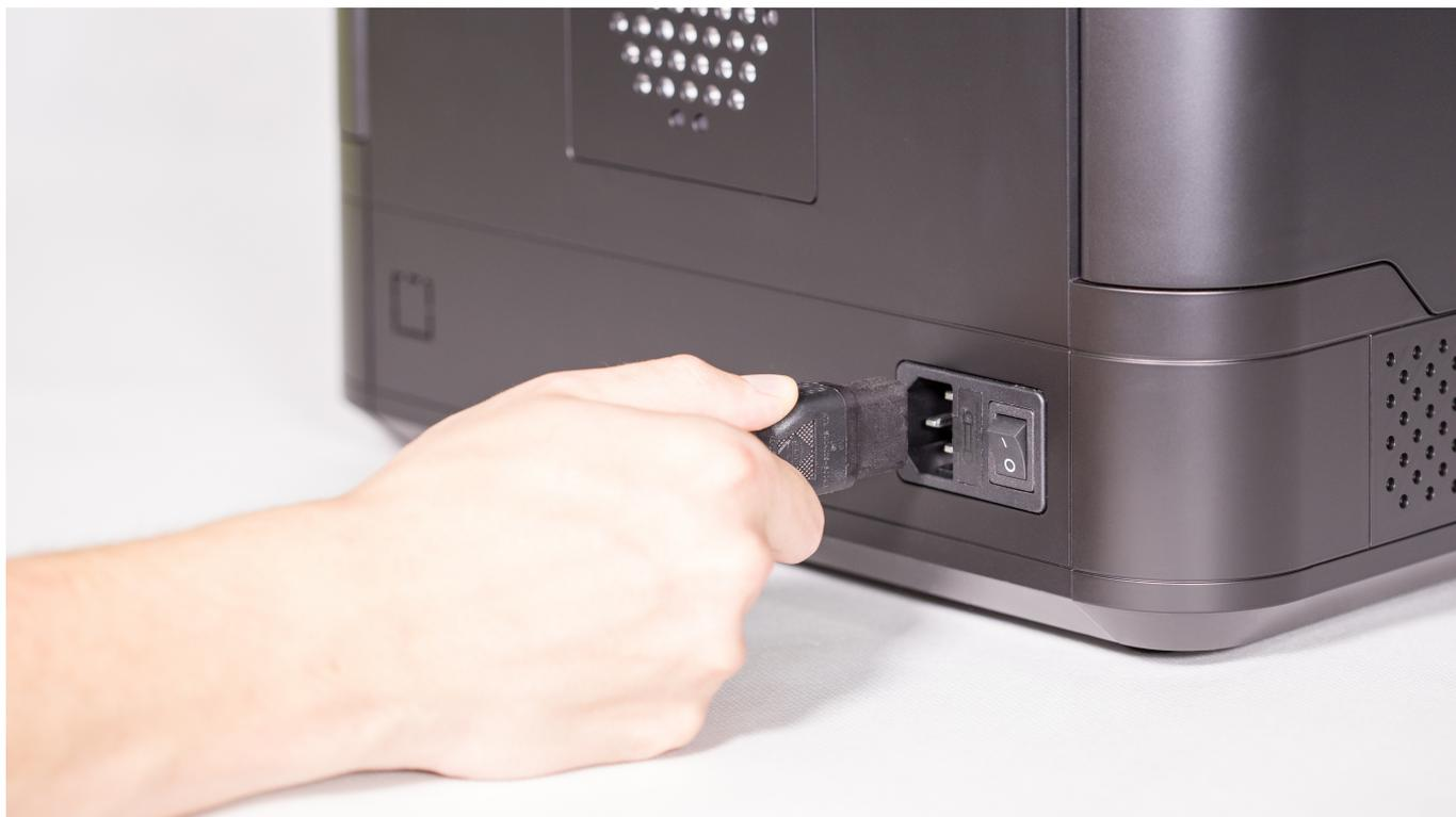
Plug in the power cable and turn on the printer.
