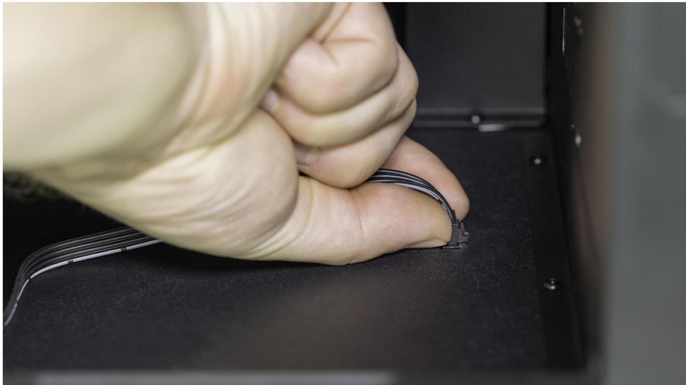
Unplug the platform cable from the bottom plate and remove the cable from the printer.
