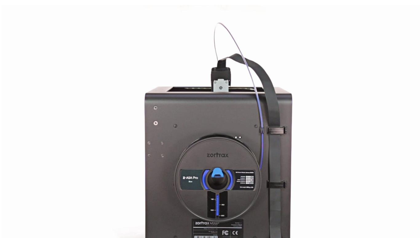
Remove the material from the material guide. Hold the end of the material and take the spool off of the spool holder.
