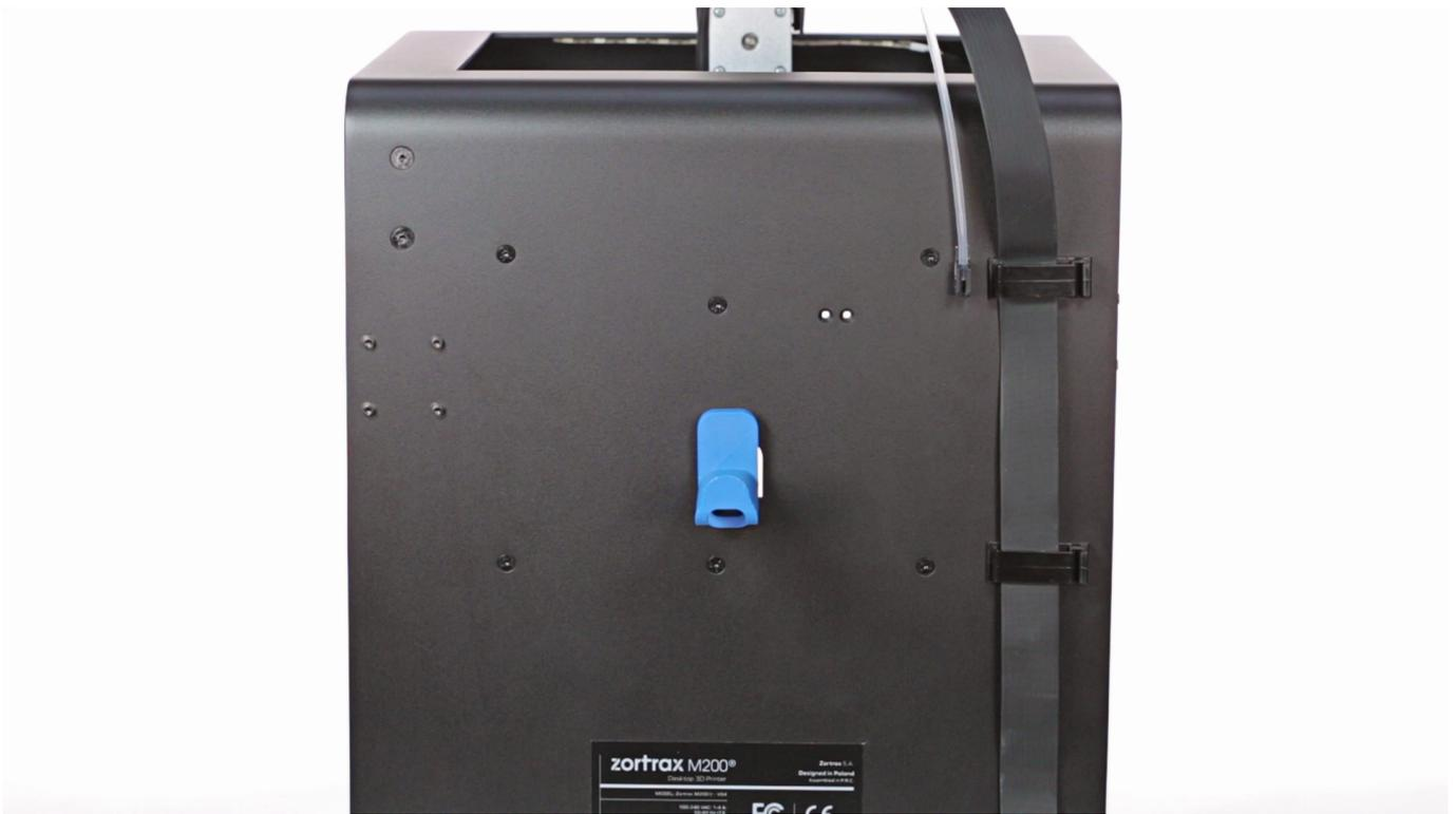
Carefully set the material spool on the holder so that the marking on the spool is visible. The spool should rotate anti-clockwise. Next, feed the material into the material guide.
