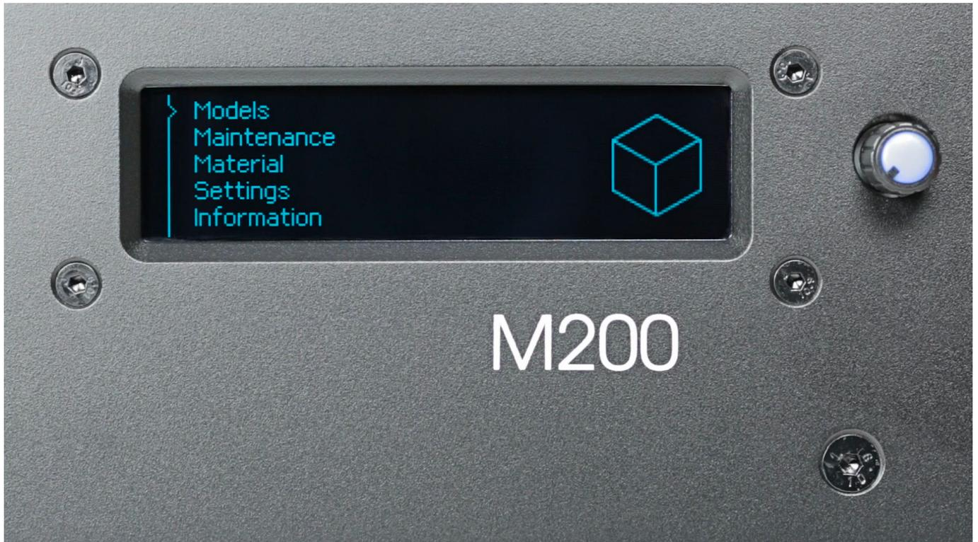
From the menu choose *Material* and then *Unload the material* option. The extruder should start to heat up automatically. Once the extruder is hot, the motor will start to unload the material.
