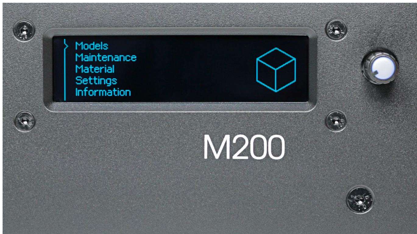
From the menu choose *Material* and then *Load the material*. At this point the printer will begin to heat up the extruder. Follow the instructions displayed on the screen.
