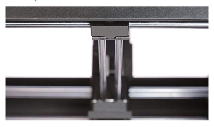
Turn the axis block and screw in the endstop sleeve using a 2mm Allen key. Turn the axis block to its previous position.
