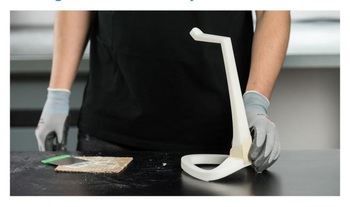
Leave the elements to dry for about 15 minutes at room temperature. Use sandpaper again to remove the excess of cured paste and clean the model with compressed air.
