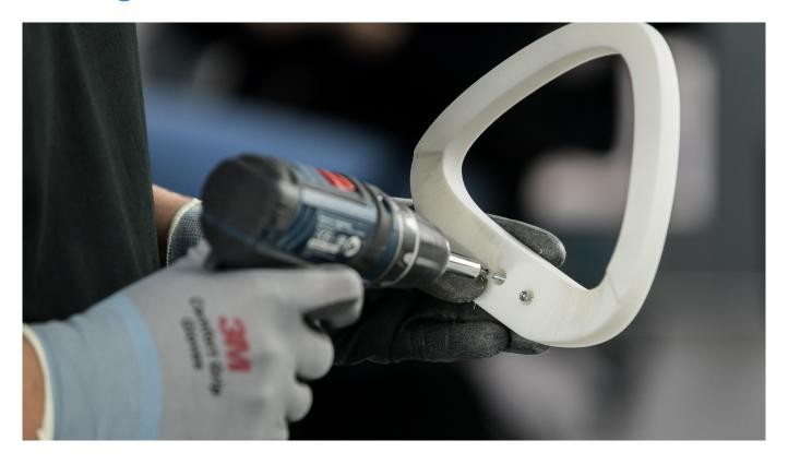
Select the right screws for the holes in the model. The screws cannot be too small because they won't fit into the holes tightly or too big as they may break the model.
