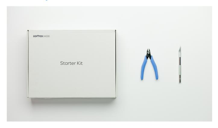
To remove the support structures from all the models, use the pliers and the scalpel provided in the Starter Kit.
