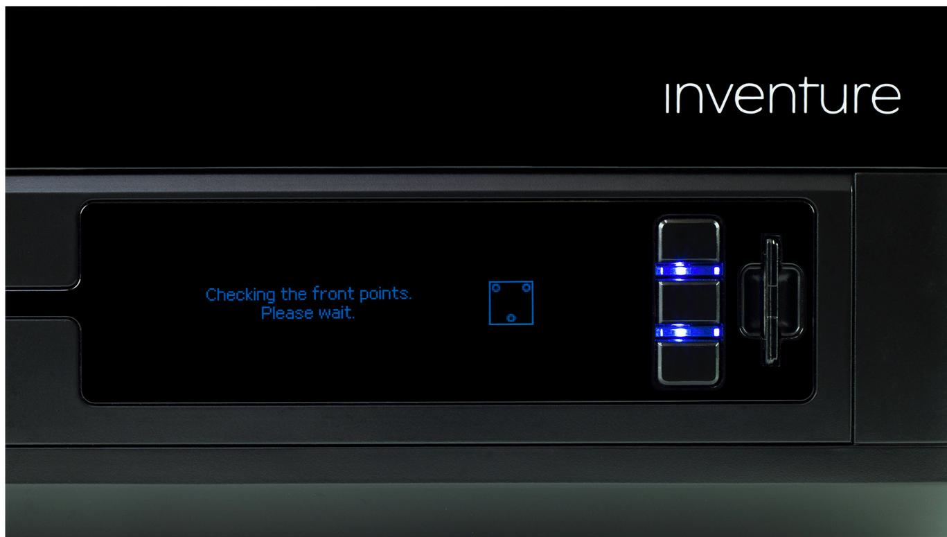
The printer will now start to check the distance between the nozzle and the points at the front and back of the platform.
