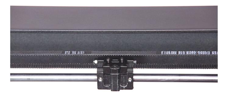
Unscrew the screw that secures the belt tensioner on each axis block and remove the belt from the block.
