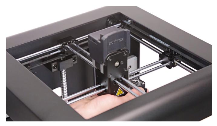
Remove the extruder along with its guide rails.
