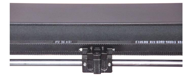
Unscrew the screw that secures the belt tensioner on each axis block and remove the belt from the block.
