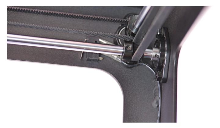
Loosen the screws on the self-aligning bearings on both sides of the X axis.
