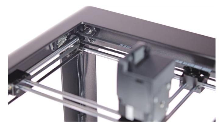
Tighten the screws that secure the self-aligning bearings on both sides of the housing.
