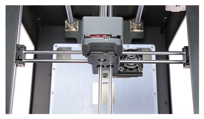
Unscrew one screw that secures the axis block cover on each block.
