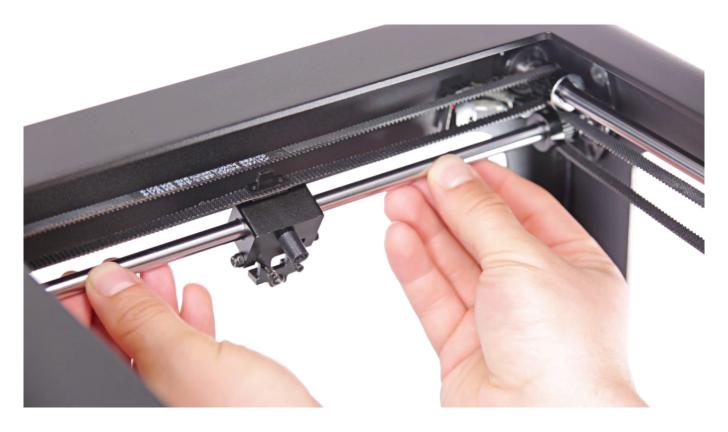
Remove the belts from the ends of the axis and remove the axis from the printer.
