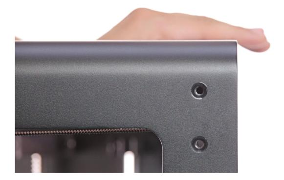
Secure the self-aligning bearings with the screws.
