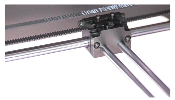
Finish tightening the screws on each axis block covers.
