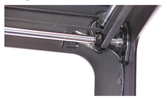
Loosen the screws on the self-aligning bearings on both sides of the X axis.
