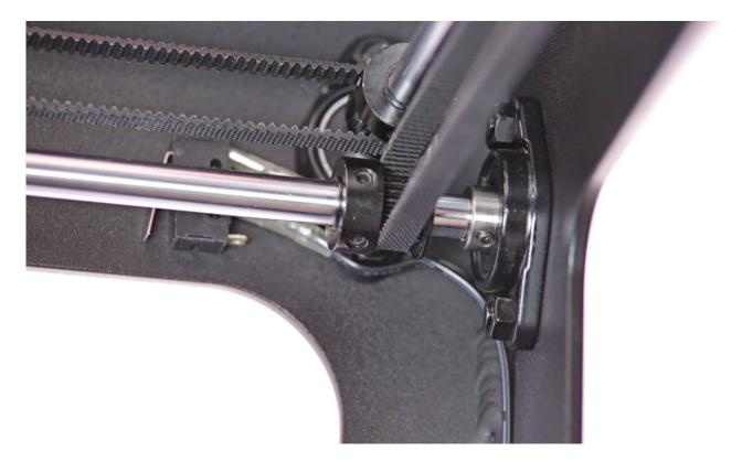
Tighten the screws on the self-aligning bearings on both sides of the X axis.
