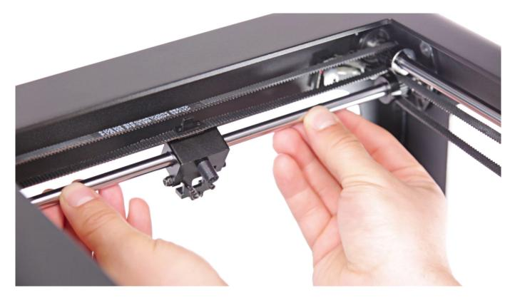
Remove the belts from the ends of the axis and remove the axis from the printer.
