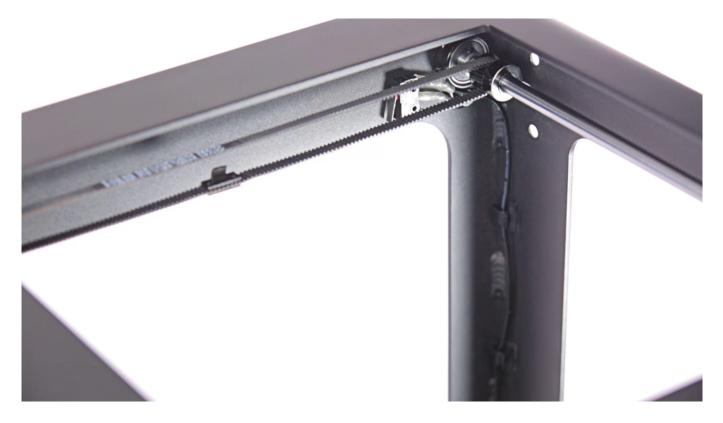
Place the new axis in the printer by putting the belts on it.
