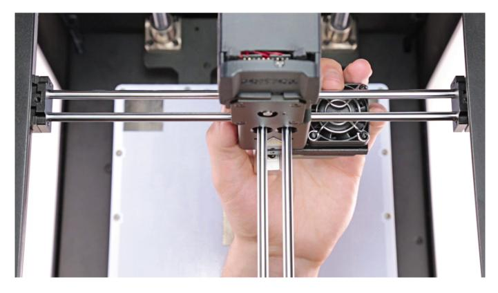
Tighten one screw that secures the axis block cover on each block.
