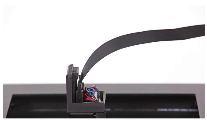
Attach the material guide to the extruder cover V2.
