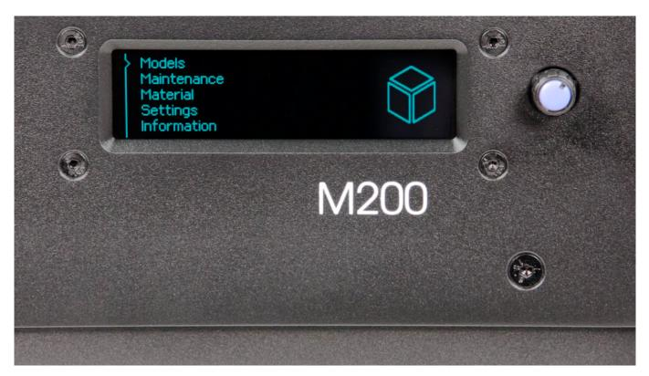
From the menu choose "Material" and then "Unload the material" option. The extruder should start to heat up automatically. Once the extruder is hot, the motor will start to unload the material.
