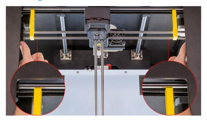
Use the jigs again to check if the extruder guide rails are parallel to the axis. If not, start again from the step no. 4.
