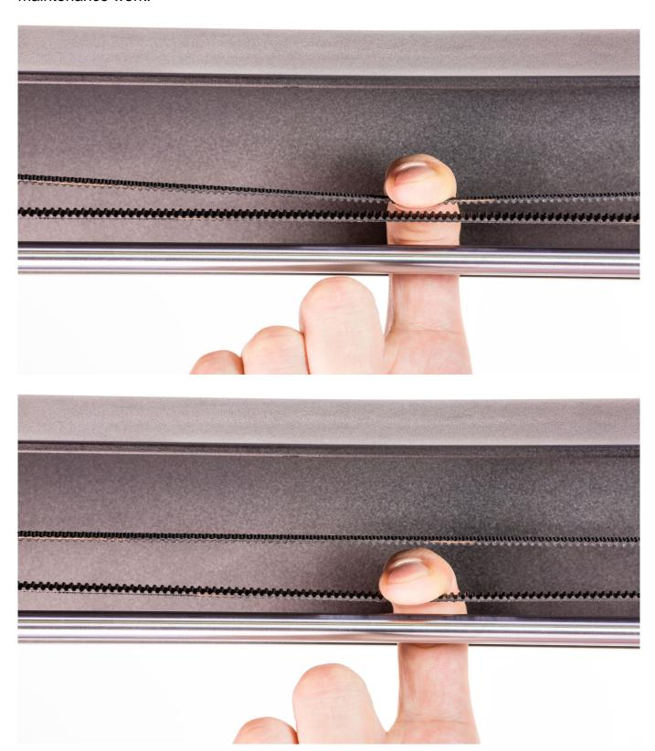
b) If not, take a piece of tape and put it on the belt. Then move the extruder manually back and forth so that the tape gets on the rack. Remove the tape.
