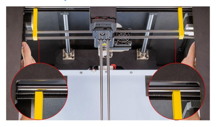
Put the jigs on the extruder guide rails and move the extruder manually so that the jigs are touching the X axis. This way, you will check if the extruder guide rails are parallel to the X axis. If not, follow the steps in this manual.
