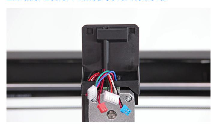
Remove the extruder lower printed cover.
