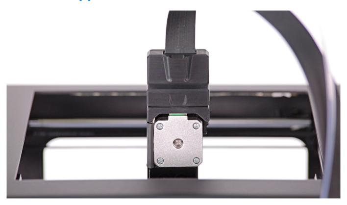
Detach the extruder upper printed cover from the extruder.
