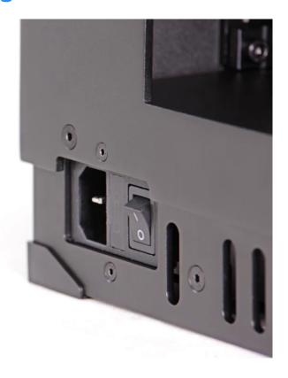
Plug the power cable in and turn on the printer.
