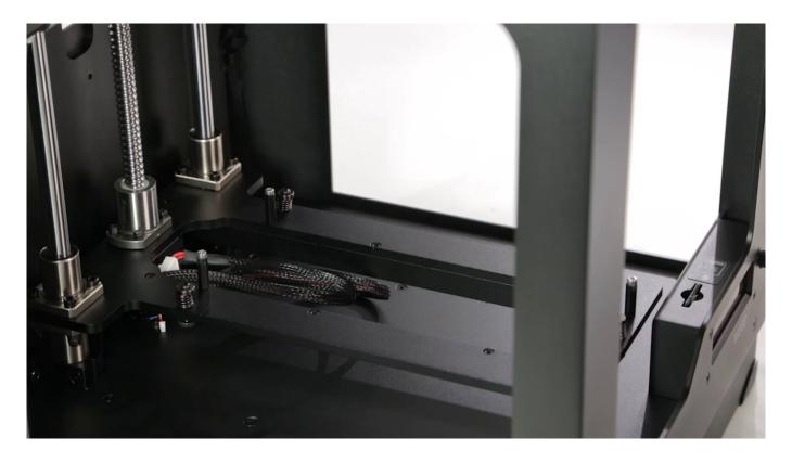
Put the platform in the printer and plug the heatbed cable in. Both big and small connectors need to be plugged in.
