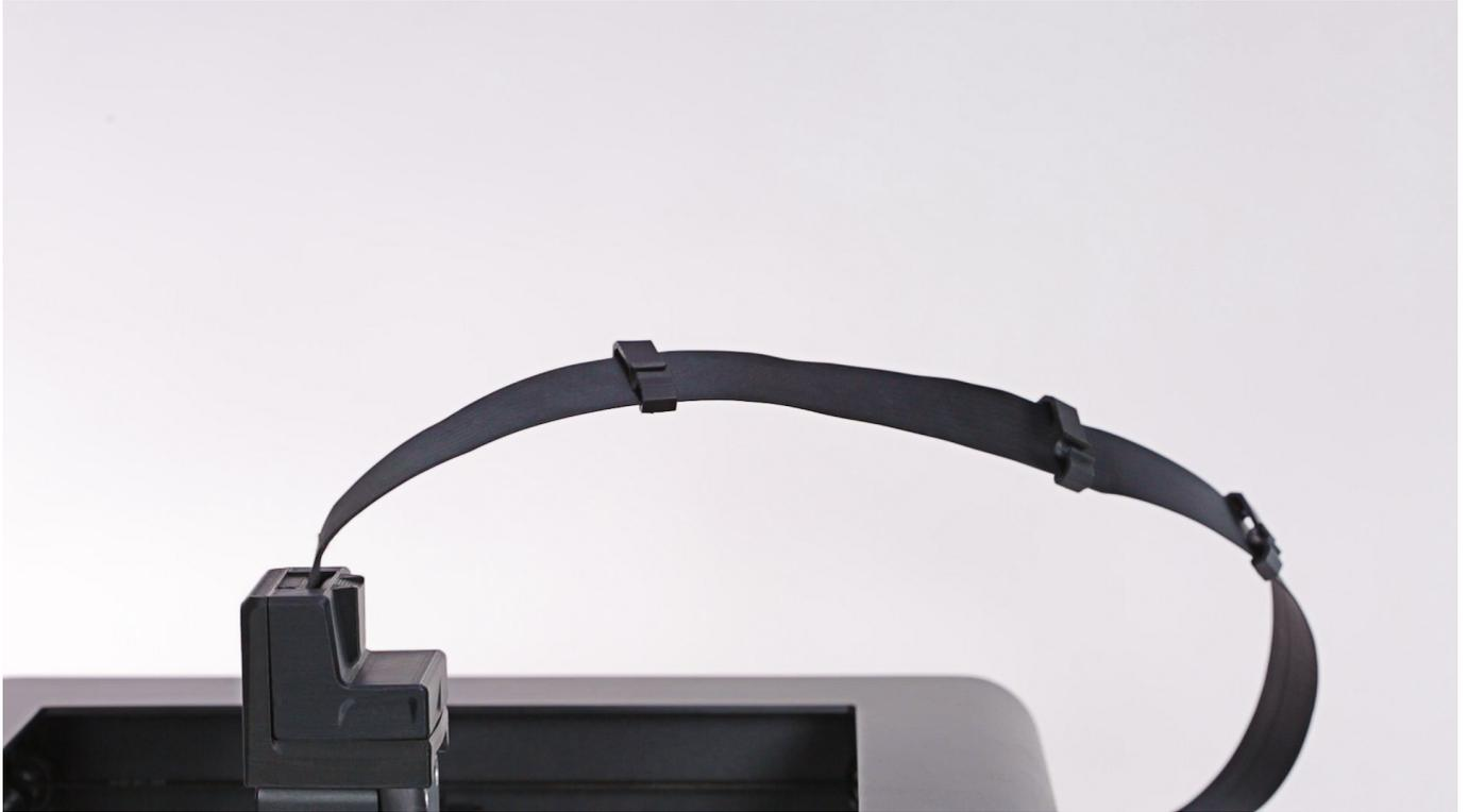
Attach the material guide to the extruder cover. Next, secure the guide to the extruder cable with the material guide clamps.
