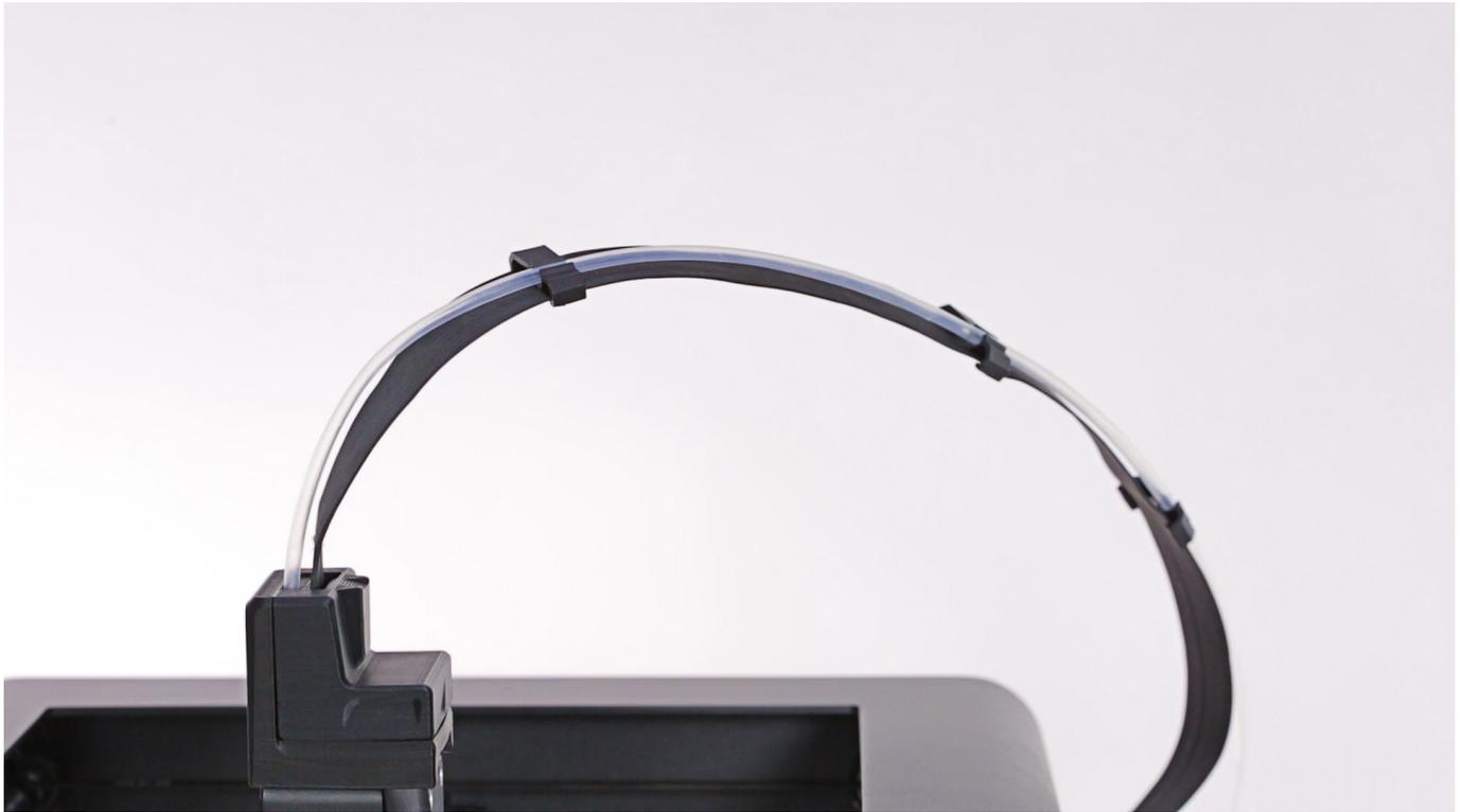
Detach the material guide from the extruder cover. Next, separate the guide from the extruder cable.
