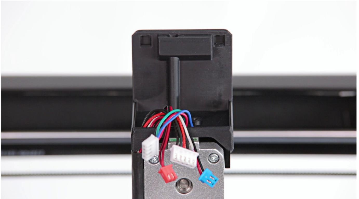
Remove the extruder lower printed cover.
