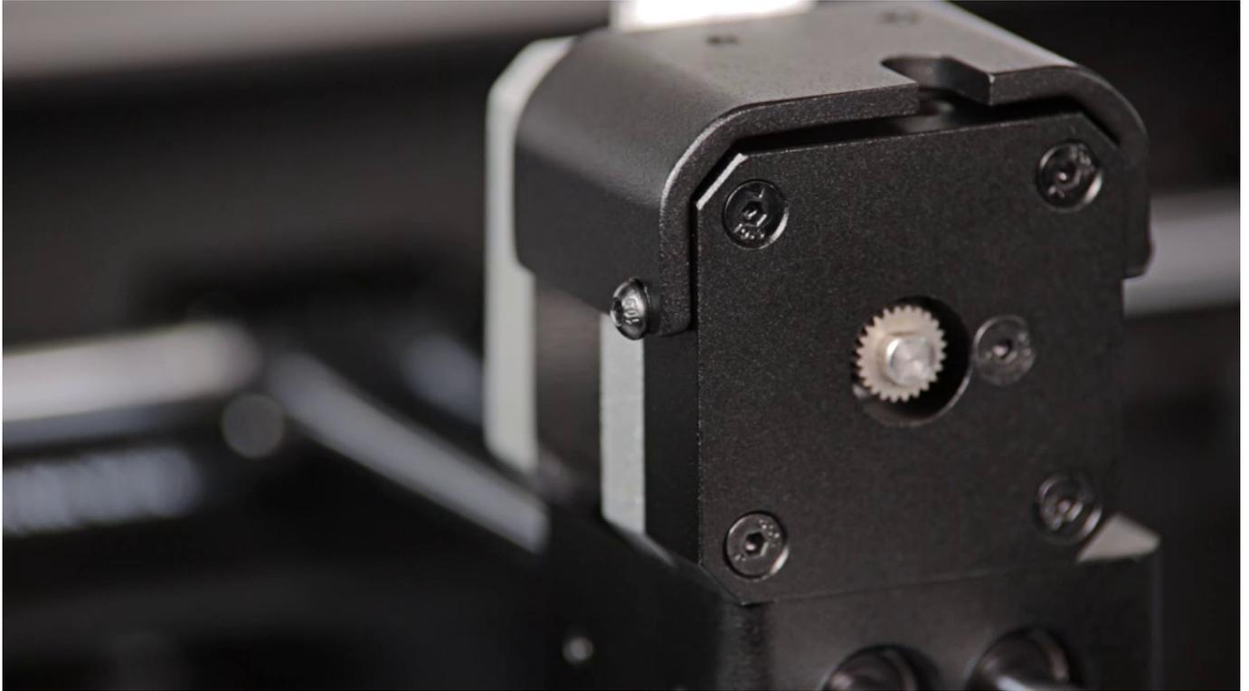
Unscrew the screws that securing the extruder aluminum cover on both sides of the extruder. Separate the cover from the extruder motor.
