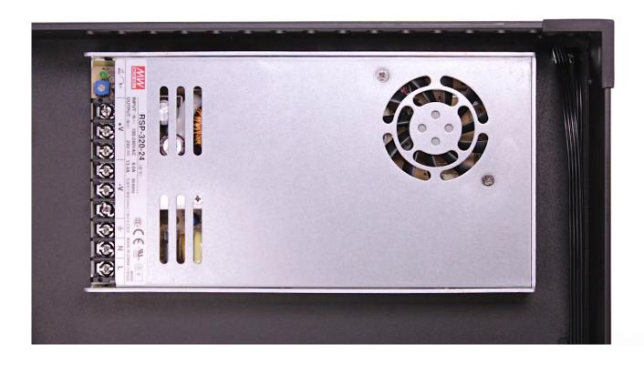
Hold the power supply unit and unscrew the four screws that secure it. Finally, remove the unit.
