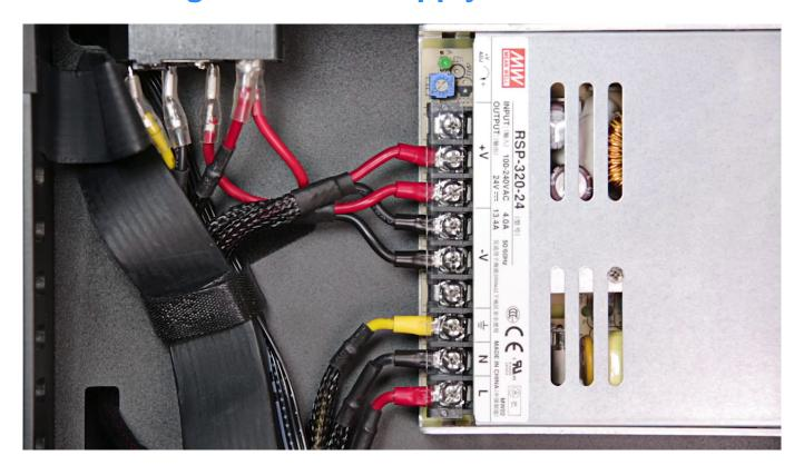
Remove the plastic cover which protects the screws that secure the power supply unit cables. Loosen the screws one by one starting from the top and remove the cables.
