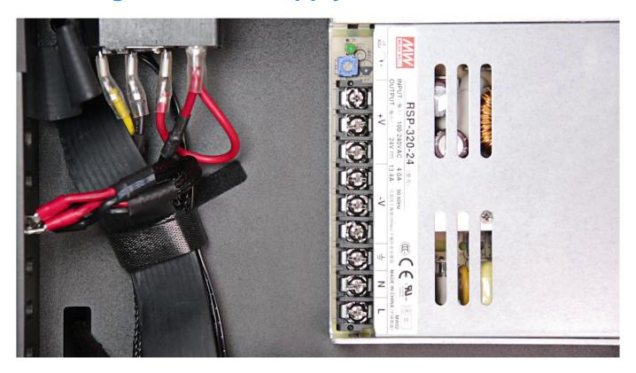
Insert the power supply unit cables into the unit and tighten each screw. Finally, reattach the plastic cover.
