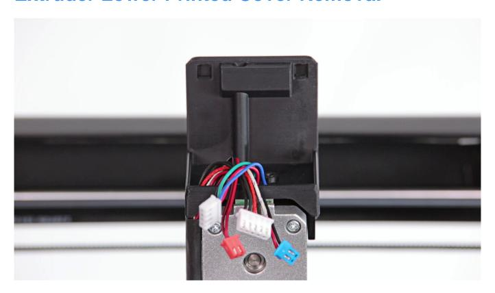
Remove the extruder lower printed cover.
