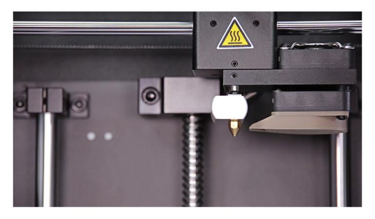
With a 1.5mm Allen key loosen the two screws that secure the hotend and remove the hotend from the extruder.
