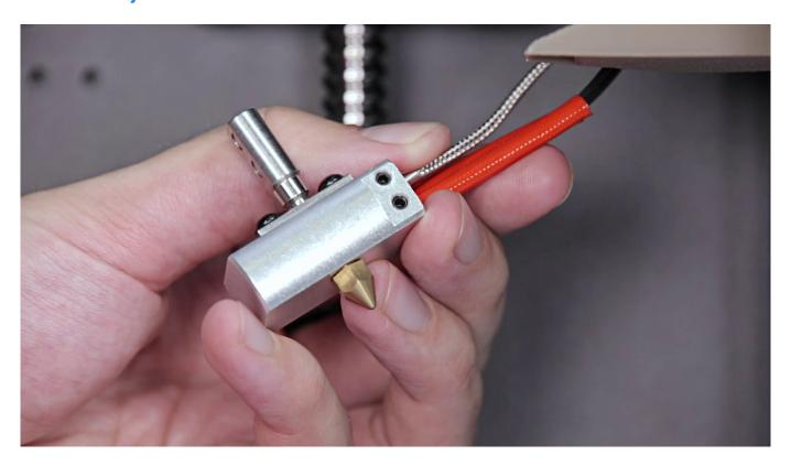
With a 1.5mm Allen key loosen the two screws that secure the heater and thermocouple in the hotend. Then remove the heater and thermocouple.
