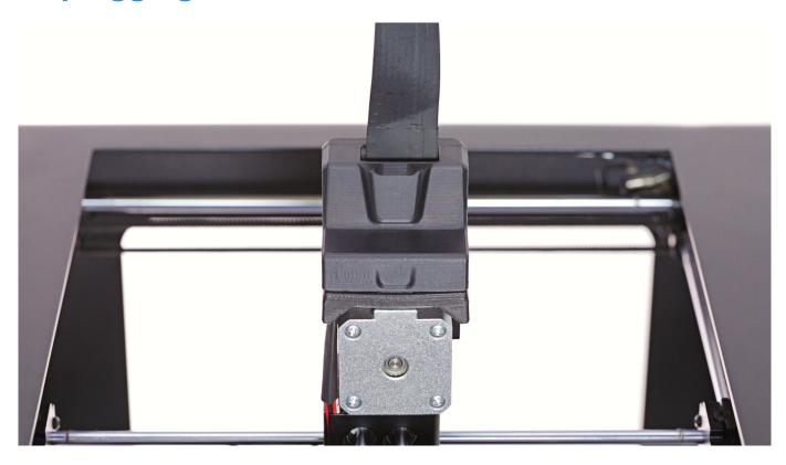
Detach the extruder upper printed cover and unplug the extruder cable.
