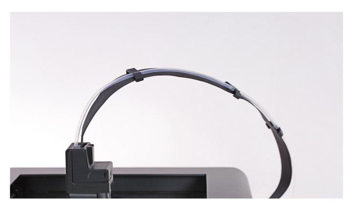
Detach the material guide from the extruder cover. Next, separate the guide from the extruder cable.
