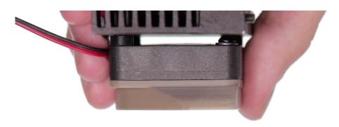
Secure the extruder lower fan with the three screws.
