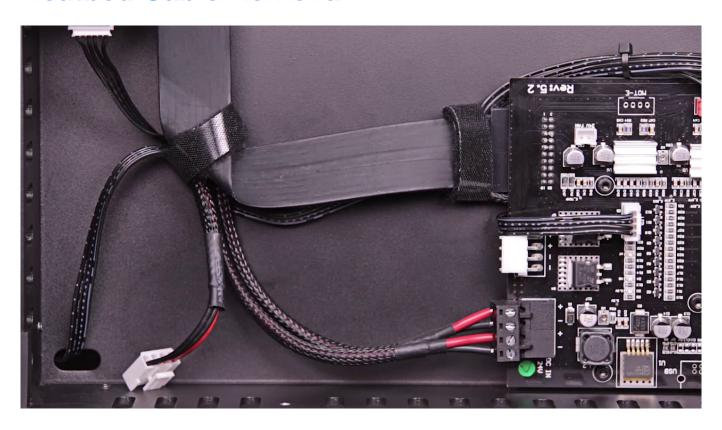
Unfasten the two extruder cable straps and carefully remove the cable from under the motherboard. Next, remove the opposite end of the cable through the hole next to the Z-axis screw.
