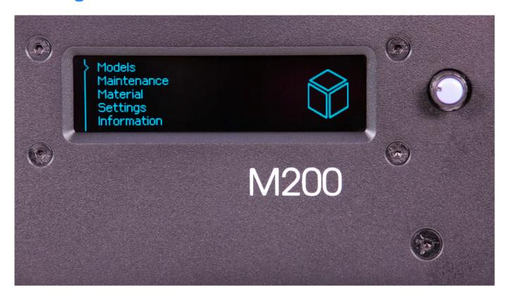
From the menu choose "Maintenance" and then "Move the platform down." Keep the knob pressed to move the platform to the very bottom.
