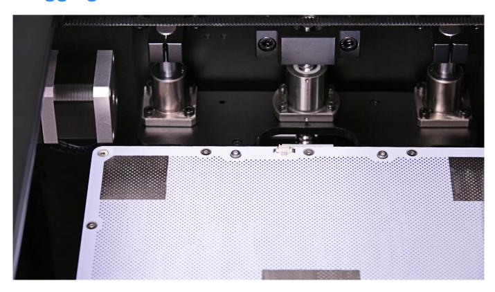
Plug the heatbed cable in. Both big and small connectors need to be plugged in.
