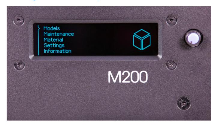
From the menu choose *Maintenance* and then *Move the platform up*. Keep the knob pressed to move the platform to the top.
