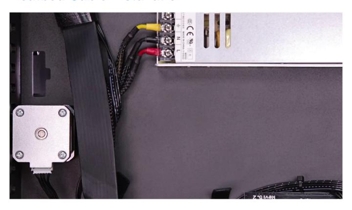
Take the new cable and pass one end (with the two connectors to be connected to the platform) through the hole next to the Z-axis screw. Pass the other end of the cable (with the two connectors to be connected to the motherboard) under the motherboard. Leave the third connector next to the motherboard.
