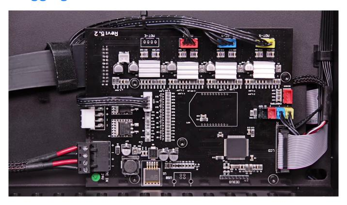
Plug the cable into the motherboard.
