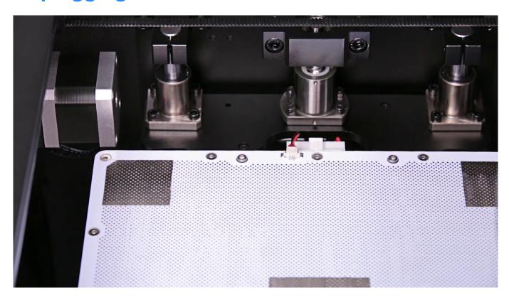
Unplug the heatbed cable from the platform. Both big and small connectors need to be unplugged.
