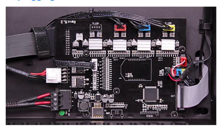
Unplug the heatbed cable from the motherboard.
