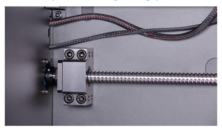
Tighten the three Z-Axis coupler screws placed on the Z-Axis side.
