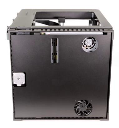
Secure the bottom plate on one side of the housing. Use a 2.5mm Allen key.
