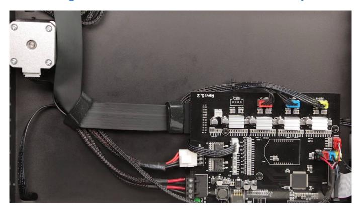
Unfasten the two extruder cable straps and unplug the cable from the motherboard. Next, unfasten the third strap. Place the extruder cable between the power supply unit and the housing. Finally, grab the cables next to the motherboard and fasten the strap.
