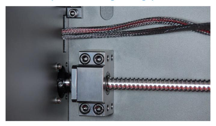
Tighten the three Z-Axis coupler screws placed on the Z-Axis coupler side.
