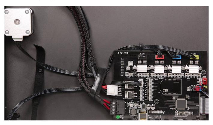
Rearrange the cables to their original position: unfasten the strap next to the motherboard. Secure the extruder cable with the first strap and plug it in. Fasten the remaining straps.
