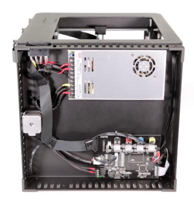
Plug the bottom fan cable into the motherboard and install the bottom plate.
