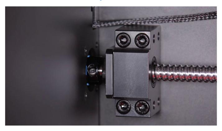
Insert the two Z-Axis motor screws in the housing, hold them and put the motor with the distance piece on them. Next, tighten the screws.
