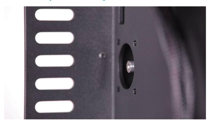
Install the Z-Axis coupler in its place and tighten the screws placed on the Z-Axis side.
