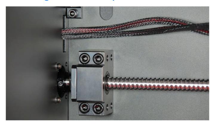
Loosen the three Z-Axis coupler screws placed on the Z-Axis motor side.
