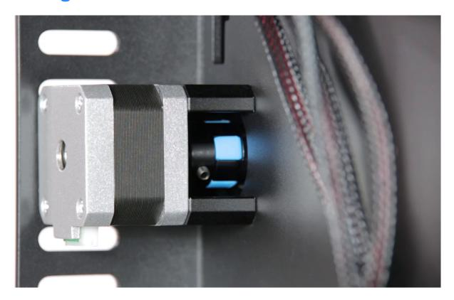
Unscrew the two screws that secure the Z-Axis motor. Remove the motor with its distance piece. Remove the two big screws from the housing.
