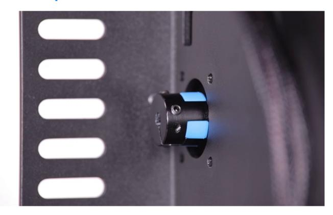
Loosen the three Z-Axis coupler screws placed on the Z-Axis side. Remove the coupler.
