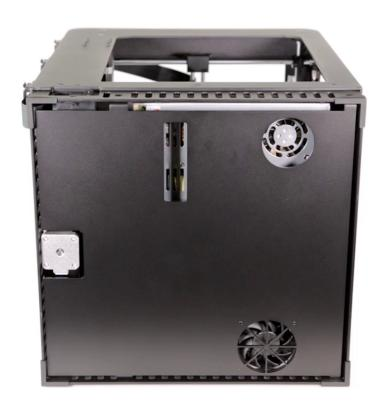
Separate the bottom plate from the printer and unplug the bottom fan cable from the motherboard.
