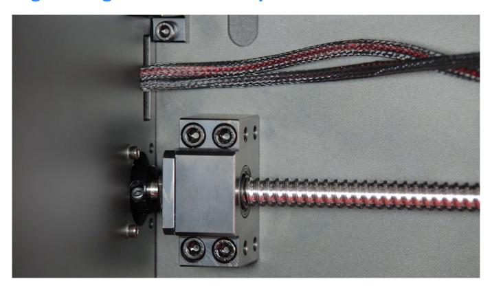
Tighten the three Z-Axis coupler screws placed on the Z-Axis motor side.
