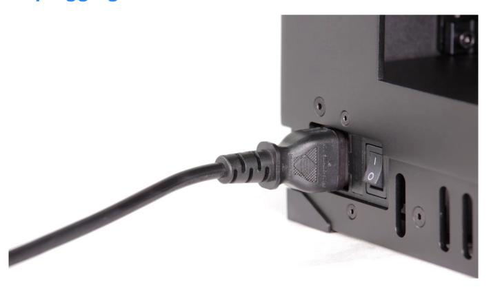
Turn off the printer and unplug the power cable. Wait a few minutes for all the capacitors to discharge.
