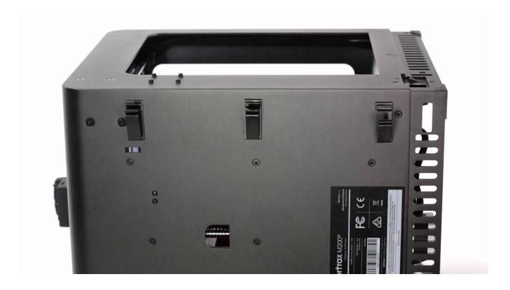
Pass the extruder cable through the hole and place in the clamps. Close the clamps. Fasten the first stap and plug the extruder cable into the motherboard. Fasten the two remaining straps.
