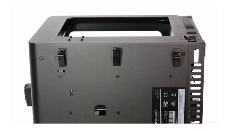
Place the cable in the cable clamps and secure it by closing the clamps. Next, pass the cable through the hole and secure it with the first strap. Plug the extruder cable into the motherboard and fasten the two remaining straps.
