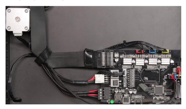
Unfasten the two extruder cable straps and unplug the cable from the motherboard. Next, unfasten the third strap. Open the three cable clamps and remove the extruder cable from the clamps, then pass the cable through the hole.
