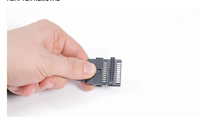
If the extruder cable you're using has an adapter, separate the adapter from the cable so you can plug it into the new version of the motherboard.
