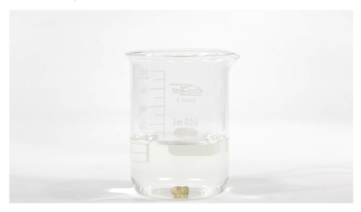
After 8-10 hours take the nozzle out of the container with pliers.
