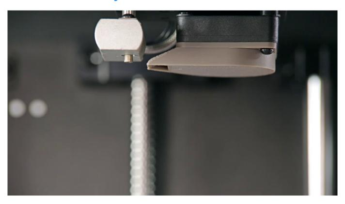
Install the nozzle in its place in the hotend and screw it in clockwise using the nozzle key (when viewed from below).
