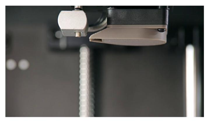
Install the nozzle in its place in the hotend and screw it in clockwise using the nozzle key (when viewed from below).
