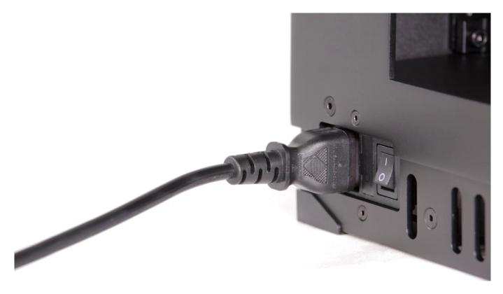
Turn off the printer and unplug the power cable. Wait about 15 minutes and let the machine cool down.
