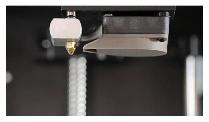
Unscrew the nozzle counterclockwise (when viewed from below). Use the nozzle key from the Starter Kit box. Removing the nozzle should take place while the extruder is still hot. When the nozzle is loose, remove it using pliers.
