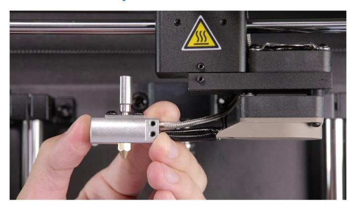
Insert the hotend into the extruder and tighten the two screws that secure it (using a 1.5mm Allen key).
