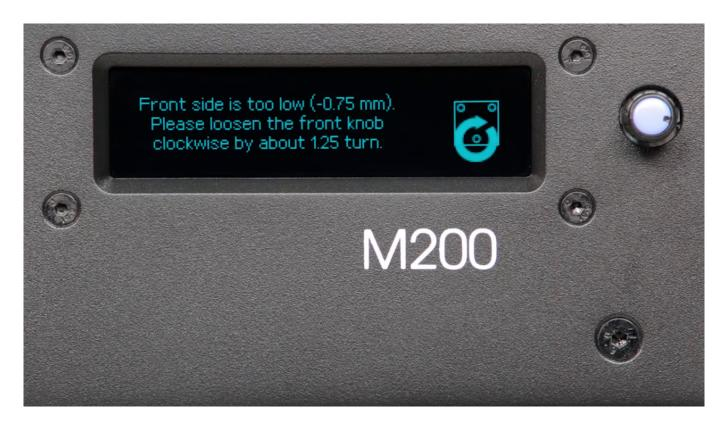
If the printer detects an incorrect distance, it will display instructions on what adjustments should be made.
