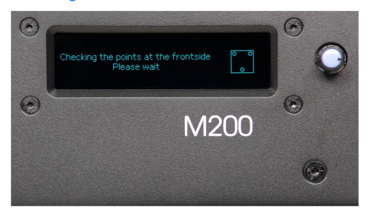
The printer will now start to check the distance between the nozzle and the points at the front of the platform.
