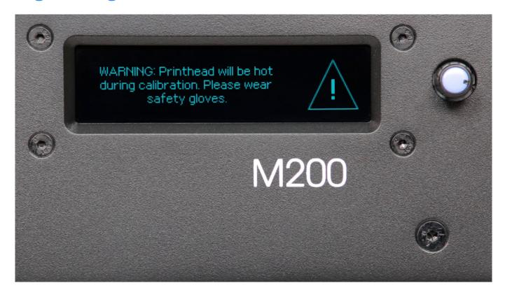
When the extruder is heated up, press the knob to start the autocalibration.
