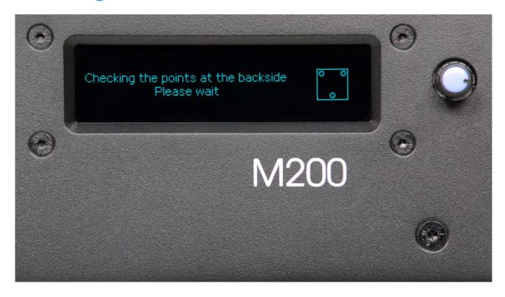
The printer will now start to check the distance between the nozzle and the points at the back of the platform.
