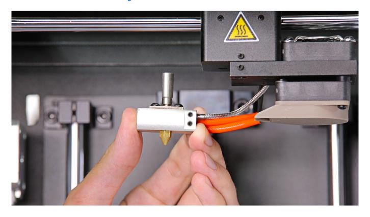
Insert the hotend into the extruder and tighten the two screws that secure it (using a 1.5mm Allen key).
