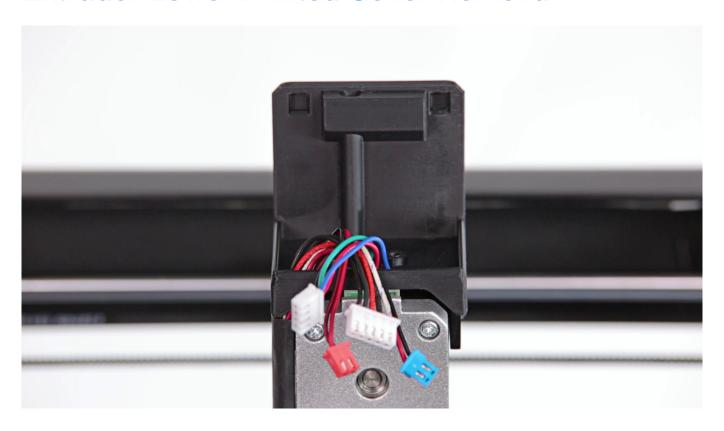
Remove the extruder lower printed cover.
