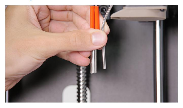
Insert the heater and thermocouple into the hotend and firmly tighten the two screws that secure them (using a 1.5mm Allen key).
