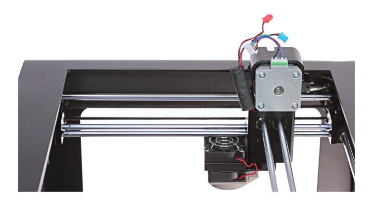
Plug the heater and thermocouple cables into the extruder PCB. Put them through the heat shrink tubing and inside the extruder's block.
