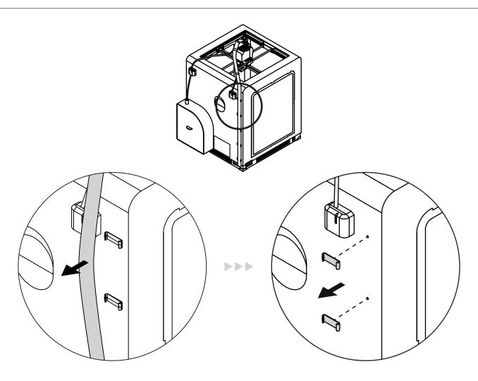
Remove the extruder cable from the clamps at the back of the printer.
