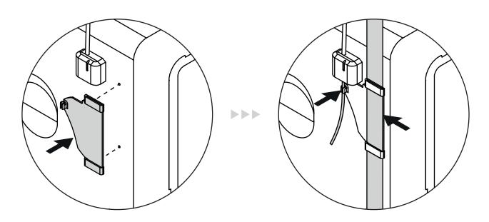
$3 \mid \text{Install the Adapter with the PTFE Tube in the printer's housing.}$
